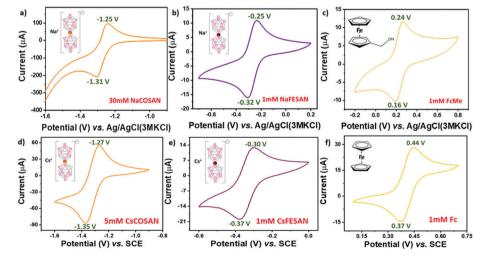
Fig. 2 Cyclic voltammograms for the reversible redox systems investigated with GC as the working electrode and Pt wire as the auxiliary electrode, measured at 100 mV s $^{-1}$ . (a) 30 mM Na[o-COSAN] in 0.3 M KNO<sub>3</sub>. (b) 1 mM Na[o-FESAN] in 0.3 M KNO<sub>3</sub>. (c) 1 mM FcMe in 0.3 M KNO<sub>3</sub>. (d) 5 mM Cs[o-COSAN] in 0.3 M TBAP/dry AcN. (e) 1 mM Cs[o-FESAN] in 0.3 M TBAP/dry AcN. (f) 1 mM Fc in 0.3 M TBAP/dry AcN.
