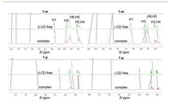
Fig. 3 Shifts of <sup>1</sup>H-NMR resonances upon binding of **1-m** (top) and **1-p** (bottom) to  $\beta$ -(left) and  $\gamma$ -CD (right).
