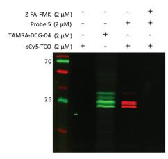
Fig. 4 Labeling of cysteine cathepsins by probe 5 in live Jurkat T-cells. Live cells were incubated with 2 µM of probe 5 for 2 hours. After incubation with probe 5, the cells were lysed and lysates were incubated with 2  $\mu$ M of sCy5-TCO for 30 minutes. Lanes were rearranged for clarity, the unprocessed gel is shown Fig. S6 (ESI†).
