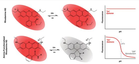
Scheme 1 Functionalization of Rhodamine 6G allows for acid-mediated transition between spirolactam (high pH) and quinone (low pH) form due to facile protonation/deprotonation of the amide substituent, resulting in dynamic "on/off" fluorescent properties.
