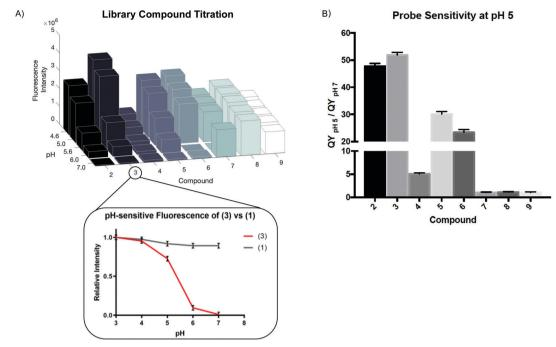
Fig. 1 Fluorescence is measured as a function of pH for each compound resulting in titration profiles, used to determine  $pK_a$  (A). Compared to unmodified starting material (1), library compounds (data for (3) shown) demonstrate an increase in fluorescence as pH decreases (A, inset). The quantum yield of each compound is calculated as the quotient of fluorescence at pH 5 compared to pH 7 (B) to determine sensitivity of our compounds.
