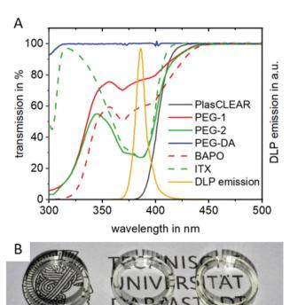
**Fig. 2** UV/VIS photospectroscopy of all resins and their single components shows the transmission of light at wavelengths between 300 and 500 nm (left *y*-axis), with the printer's DLP emission spectrum (right *y*-axis) showing a clear peak at 385 nm (A). Images of printed cell culture dishes of all printing materials show the high post-printing transparency for all three selected resins (B).
