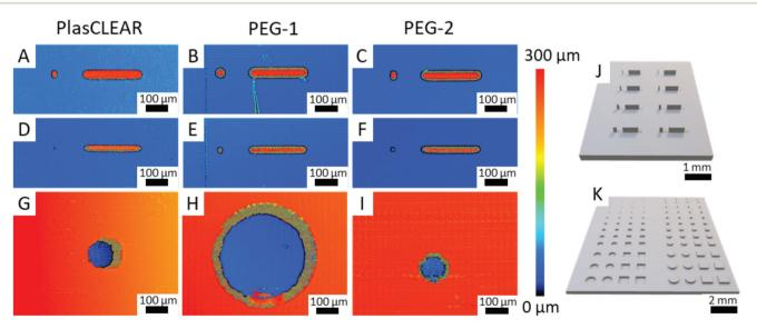
Fig. 7 CLSM height images of printed pillars, walls (A-F) and holes (G-I). With all three resin, a minimum pillar size of 50 µm (A-C), and minimum wall size of 35 µm (D and E) could be printed. Minimum hole size varies with resin, and is 120 µm for PlasCLEAR (G), 370 µm for PEG-1 (H) and 100 µm for PEG-2 (I). CAD models for testing the maximum resolution for freestanding pillars and walls (J) and holes (K).
