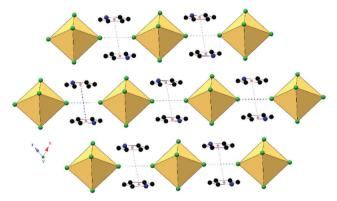
Fig. 3 Packing of 1, viewed along the b-axis, showing end to end halogen bonding (black dashed lines) between octahedra and  $\pi \cdots \pi$  stacking (blue dashed lines) between pyridinium cations. Red spheres represent centroids of pyridinium rings.
