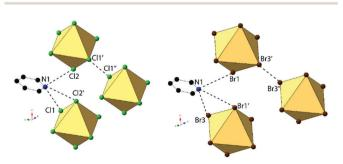
**Fig. 2** Local structure of isomorphous compounds **1** (left) and **5** (right) showing halogen bonding between adjacent  $[TeX_6]^{2-}$  octahedra and trifurcated hydrogen bonding between the pyridinium cation and two  $[TeX_6]^{2-}$  octahedra.
