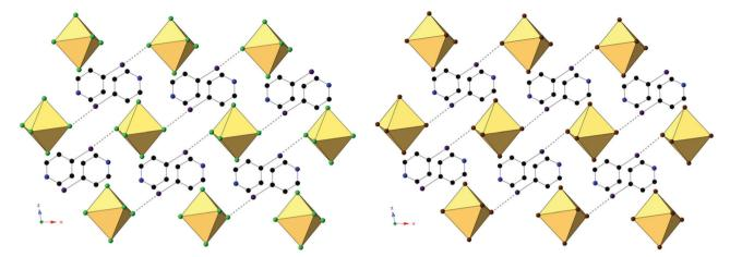
Fig. 9 Packing of 4 (left) and 8 (right) as seen directly along the b-axis, showing halogen bonding (black dashed lines) between pyridinium halogens and [TeX<sub>6</sub>]<sup>2-</sup> octahedra.
