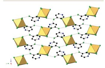
Fig. 5 Packing of 2 highlighting the extended halogen bonding (dashed lines) between [TeCl<sub>6</sub>]<sup>2-</sup> octahedra and associated ClPy cations.
