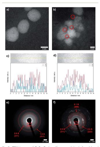
Fig. 7 TEM images of  $CoFe_2O_4$  (x = 1) nanoparticles before (a) and after OER (b), TEM-EDX linescans on a single particle for  $CoFe_2O_4$  (x =1) before (c) and after electrochemical treatment (d) and SAED patterns after OER measurements for  $Co_x Fe_{3-x}O_4$  with x = 2.25 (e) and 2.50 (f).
