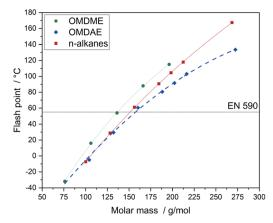
Fig. 11 Flash points of OMDAEs compared to OMDMEs and n-alkanes with similar molar mass. Data points and trend lines for OMDMEs (green) and n-alkanes (red) as well as data points and values predicted by the regression function for OMDAEs (blue).
