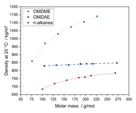
Fig. 7 Densities of OMDAEs compared to OMDMEs and n-alkanes with similar molar mass. Data points and trend lines for OMDMEs (green) and n-alkanes (red) as well as data points and values predicted by the regression function for OMDAEs (blue).
