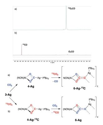
Fig. 9  $^{13}$ CO<sub>2</sub> 'crossover' labelling experiments (and their associated spectra) carried out with 4-Ag and 4-Ag- $^{13}$ C: (a) addition of  $^{13}$ CO<sub>2</sub> to 4-Ag to yield 6-Ag- $^{13}$ C and CO; (b) addition of unlabelled CO<sub>2</sub> to 4-Ag- $^{13}$ C to yield 6-Ag and  $^{13}$ CO.
