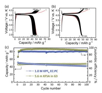
Fig. 5 Galvanostatic charge-discharge curves of KVPP electrodes in K cells filled with different electrolytes at C/20 rate in 2.0-4.5 V: (a) 1 mol  $dm^{-3}$  KPF<sub>6</sub>/EC : PC (1 : 1 v/v) electrolyte and (b) 5.6 mol kg<sup>-1</sup> KFSA/ triglyme (G3) electrolyte. (c) Comparison of discharge capacity and coulombic efficiency of the two different electrolyte cells
