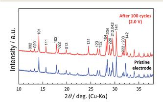
Fig. 4 Comparison of XRD patterns of pristine KVPP electrode and the KVPP electrode in the discharged state at  $2.0~\rm V$  at the  $100^{\rm th}$  cycle.
