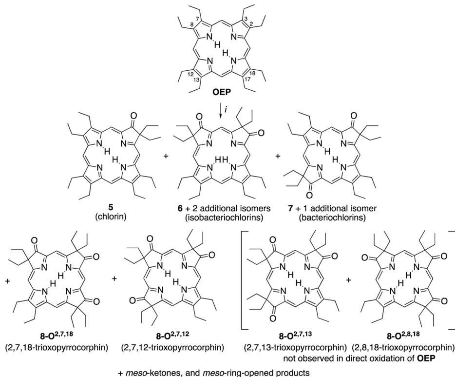
**Scheme 2** Oxidation of octaethylporphyrin OEP to the corresponding  $\beta$ -oxo derivatives.<sup>10a,15</sup> Reaction conditions: (i) (1) H<sub>2</sub>O<sub>2</sub> (3%)/H<sub>2</sub>SO<sub>4</sub> (96%), ~15 min, 0 °C. (2) NaOAc, H<sub>2</sub>O. (3) Chromatography. The atom numbering in octaethylporphyrin OEP shows the numbering system used, the basis for the  $\beta$ -ketone names.
