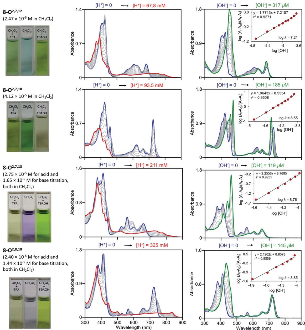
Fig. 7 UV-vis titration of triketone isomers **8** indicated; acid titration using TFA (left column) and base titration using TBAOH (right column) in the  $[\text{H}^+]/[\text{OH}^-]$  ranges indicated. The photographic images on the left show the colours of the solutions at their start and end points, see ESI†
