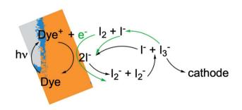
Fig. 10 Schematic of the electrolyte reactions involved in reduction of Dye $^+$ . The paths indicated by black arrows correspond to Sc3. The green arrows show how the  $I_2$ -electron recombination reactions from Sc1 and Sc2 are coupled to them.
