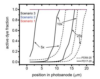
Fig. 8 Profiles of the fraction of dyes that are photoactive within the pores for Sc1 and Sc2, which allow electrolyte–electron recombination, and Sc3, which does not, as a function of excitation frequency. The active dye fraction at 1× excitation frequency is 1.0 everywhere in the photoanode for both architectures and all 3 scenarios.
