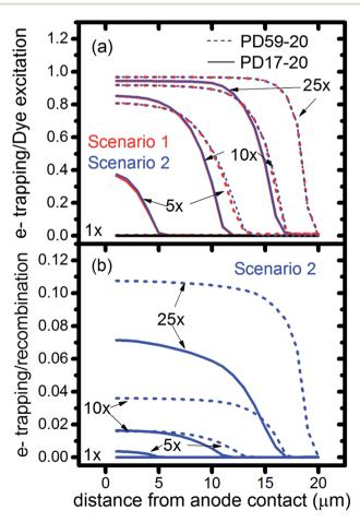
Fig. 7 Ratios of cumulative events as a function of position in the photoanode after 0.8 s, as monitored by markers in the reaction steps. (a) Electron recombination with I $_2$  relative to dye excitation for Sc1 and Sc2, (b) electron recombination with I $_2$  relative to interfacial formation of I $_3$ <sup>-</sup> from I $_2$  and I $^-$ .
