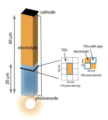
Fig. 2 Schematic of the model architecture using the color scheme from Fig. 1. The photoanode is represented using a single pore surrounded by stacks of 10 nm  $\times$  10 nm  $\times$  10 nm TiO<sub>2</sub> nanoparticles that are coated with dye, filled with electrolyte and in contact with bulk electrolyte. Two limiting pore architectures are considered, and their cross-sectional structure is shown
