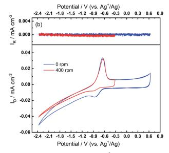
Fig. 7 RRDE measurements at 100 mV s<sup>-1</sup> with rotation speeds of 0 rpm and 400 rpm (a) before and (b) after the oxidation peak appears in  $O_2$ -bubbled 0.1 M TBAClO<sub>4</sub>/0.01 M Ca(ClO<sub>4</sub>)<sub>2</sub>/DMSO. The disc and ring electrodes are GC and Pt, respectively, and the potential of ring is -0.37 V. A potential limit of -2.37 V is set in (b), in accordance with previous CVs wherein the reversible OER peak can be found.
