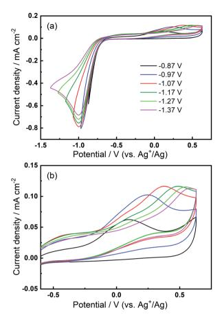
Fig. 8 (a) Cyclic voltammograms on Au and (b) the magnified OER region at 100 mV s $^{-1}$  within a reduced potential window (lower limit expanding from -0.87 V to -1.37 V) in O<sub>2</sub>-saturated 0.1 M TBAClO<sub>4</sub>/0.01 M Ca(ClO<sub>4</sub>)<sub>2</sub>/DMSO.
