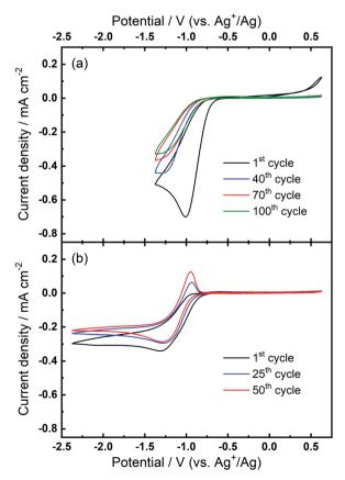
Fig. 5 Comparative cyclic voltammograms of the ORR and OER on Au at 100 mV s $^{-1}$  within (a) the reduced potential window (-1.37 V to 0.63 V) and, subsequently, (b) the expanded potential window (-2.37 V to 0.63 V) in O<sub>2</sub>-saturated 0.1 M TBAClO<sub>4</sub>/0.01 M Ca(ClO<sub>4</sub>)<sub>2</sub>/DMSO.
