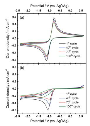
Fig. 1 (a) Cyclic voltammograms of the ORR and OER on an Au electrode at 100 mV s $^{-1}$  in O $_2$ -saturated (a) 0.1 M TBAClO $_4$ /DMSO and (b) 0.1 M Ca(ClO $_4$ ) $_2$ /DMSO.
