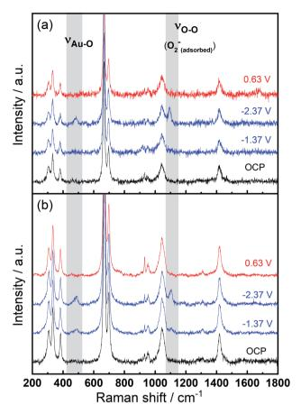
Fig. 6 In situ SERS (normalised) measured at various potentials on a roughened Au electrode in  $O_2$ -saturated (a) 0.1 M TBACl $O_4$ /0.01 M Ca(Cl $O_4$ )<sub>2</sub>/DMSO and (b) 0.1 M TBACl $O_4$ /DMSO.
