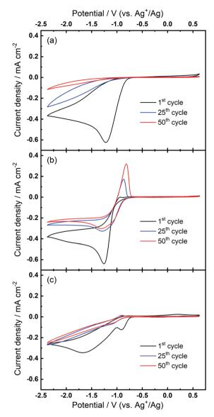
Fig. 4 Comparative cyclic voltammograms of the ORR and OER on Au at 100 mV s<sup>-1</sup> in O<sub>2</sub>-saturated electrolytes of (a) Electrolyte 1 (0.01 M  $Ca(ClO_4)_2/DMSO)$ , (b) Electrolyte 2 (0.1 M TBAClO<sub>4</sub>/0.01 M Ca(ClO<sub>4</sub>)<sub>2</sub>/ DMSO) and (c) Electrolyte 1 again. All CVs were measured using the same electrode
