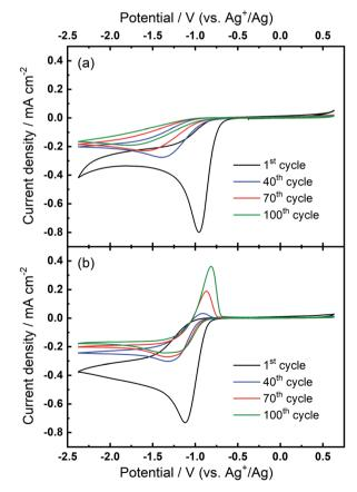
Fig. 2 Cyclic voltammograms of the ORR and OER on Au at 100 mV s $^{-1}$  in O $_2$ -saturated (a) 0.1 M TBAClO $_4$ /0.1 M Ca(ClO $_4$ ) $_2$ /DMSO and (b) 0.1 M TBAClO $_4$ /0.01 M Ca(ClO $_4$ ) $_2$ /DMSO.
