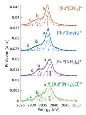
Fig. 3  $\,$  4d  $\rightarrow$  2p emission (VtC XES, solid line) measured at an incident energy above the ionization threshold of the L<sub>3</sub>-edge (2950 eV). The dashed lines are the TDDFT calculated spectra, obtained by convolving the discrete transitions (vertical sticks) with 1.5 eV (FWHM) Lorentzian function. A global shift of 96.3 eV is applied to the calculated spectra.
