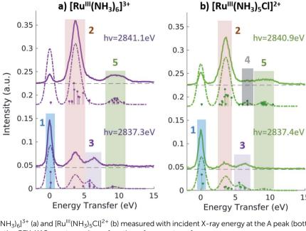
Fig. 5 2p4d RIXS of  $[Ru^{III}(NH_3)_6]^{3+}$  (a) and  $[Ru^{III}(NH_3)_5CI]^{2+}$  (b) measured with incident X-ray energy at the A peak (bottom panels) and B peak (top panels) peak of the respective PFY-XAS spectra and as a function of energy transfer.
