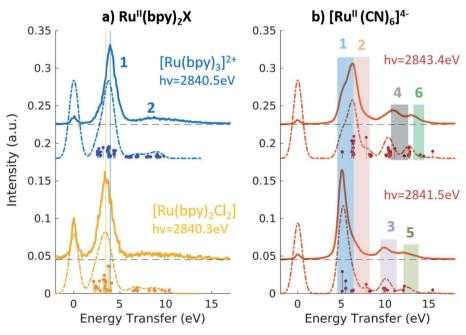
Fig. 4 (a) 2p4d RIXS of  $[Ru^{II}(bpy)_3]^{2+}$  (top) and  $[Ru^{II}(bpy)_2Cl_2]$  (bottom) measured with incident X-ray energy at the B peak of the PFY-XAS spectra and as a function of energy transfer. (b) 2p4d RIXS of  $[Ru^{II}(CN)_6]^{4-}$  measured with incident X-ray energy at the B peak (bottom) and at the C peak (top) of the PFY-XAS spectra and as a function of energy transfer.
