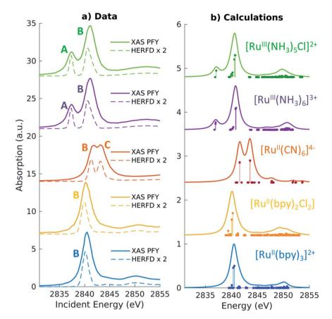
Fig. 2 (a) Measured Partial Fluorescence Yield (PFY, solid lines) absorption and High Energy Resolution Fluorescence Detected (HERFD, dashed lines) absorption for the Ru model complexes investigated in our study. (b) TDDFT calculated  $L_3$ -edge XAS spectra. The vertical lines represent discrete excitations (core-excited states), which have been convolved with 1.5 eV (FWHM) Lorentzian functions to generate the spectra (solid lines). A global shift of 2.3 eV is applied to the calculated spectra.
