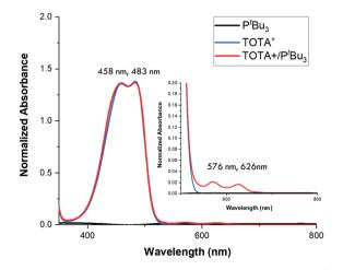
Fig. 3 Normalized UV-vis spectra of TOTA<sup>+</sup> (blue trace,  $1\times10^{-5}$  M in CH<sub>2</sub>Cl<sub>2</sub>), P<sup>t</sup>Bu<sub>3</sub> (black trace,  $1\times10^{-5}$  M in CH<sub>2</sub>Cl<sub>2</sub>), and a 1 : 1 mixture of P<sup>t</sup>Bu<sub>3</sub>/TOTA<sup>+</sup> (red trace, both substrates  $1\times10^{-5}$  M in CH<sub>2</sub>Cl<sub>2</sub>).
