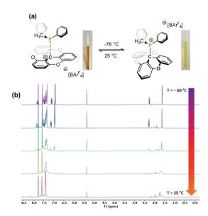
Fig. 2 (a) Reversible Lewis adduct formation between TOTA $^+$  and PPh $_2$ Me. (b) Variable temperature (VT) 500 MHz  $^1$ H NMR spectra of TOTA $^+$  (12 mg, 0.01 mmol) and PPh $_2$ Me (4.2 mg, 0.02 mmol) in CD $_2$ Cl $_2$  indicating formation Lewis adduct at  $-60\,^{\circ}$ C.
