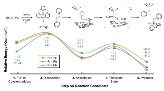
Fig. 5 Reaction coordinate for the activation of  $(SPh)_2$  using  $[TOTA-PR_3]^+$  (R =  $^tBu$ , Ph, or Me) adducts. All models were calculated using the CAM-B3LYP functional, 6-311G(d,p) basis set, SCRF PCM acetonitrile solvation model, and Grimme D3 empirical dispersion damping functions. Transition states were found with a single imaginary frequency and as local maxima by IRC calculations.
