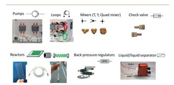
Fig. 2 Flow equipment and representation.
