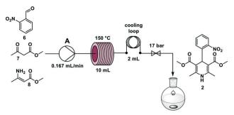
Fig. 4 Continuous flow synthesis of nifedipine 2 in a Vapourtec R2 pump module using one feed (A) and a stainless-steel reactor coil (10 mL, i.d. 0.8 mm) heated by a Vapourtec R4 module.
