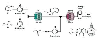
Fig. 5 Continuous flow synthesis of lidocaine 3. First step: two feeds (A and B), are mixed in a T-junction and reacted at room temperature in a 1.6 mL PFA coil (i.d. 0.8 mm). Second step: the solution exiting the first reactor is combined with a third feed (C) and passes through a stainless-steel reactor (i.d. 0.8 mm) at 130 °C.
