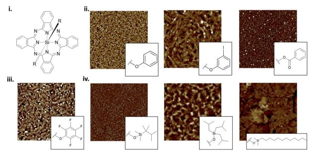
Fig. 13 (i) Structure of axially substituted  $R_2$ -SiPc. AFM images of  $R_2$ -SiPcs with (ii) phenoxy, (iii) pentafluorophenoxy and (iv) alkyl axial substituents. Adapted with permission from (ii) ref. 130, (iii) ref. 131, and (iv) ref. 132. Copyright© 2020 American Chemical Society. Copyright© 2019 Wiley-VCH Verlag GmbH & Co. KGaA.
