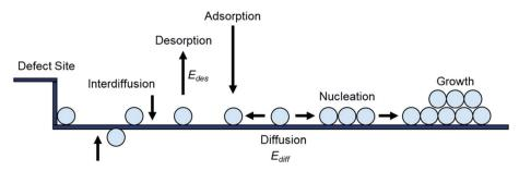
Fig. 2 Schematic diagram of nucleation and growth processes on a substrate
