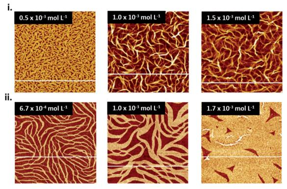
Fig. 8 AFM images ( $5 \mu m \times 5 \mu m$ ) of CuPc thin-films fabricated by (i) spin coating and (ii) dip coating at various concentrations of CuPc solution on SiO<sub>2</sub> substrates. (i) Adapted with permission from ref. 79. Copyright© 2020 the Authors under the Creative Commons Attribution Non-Commercial No Derivatives 4.0 License. (ii) Adapted with permission from ref. 80. Copyright© 2015 Elsevier B. V.
