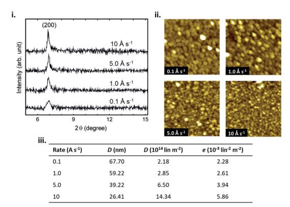
Fig. 5 (i) XRD pattern of CuPc thin-films, (ii) AFM images (1  $\mu$ m  $\times$  1  $\mu$ m) of CuPc thin-films, and (iii) crystal size (*D*), dislocation density (*d*) and lattice microstrain (e) of CuPc thin-films, deposited at various deposition rates. Adapted with permission from ref. 40. Copyright © 2012 Elsevier Ltd.
