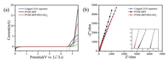
(a) LSV curves and (b) impedance spectra of the Celgard 2325 separator absorbed liquid electrolyte and PVDF-HFP-based GPEs.
