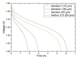
Fig. 4 Static self-discharge curves of Aemion (50 μm), Aemion+ (50  $\mu$ m), Aemion+ (15  $\mu$ m) and Nafion 212 (50  $\mu$ m) in a diluted (0.1 M) vanadium electrolyte.
