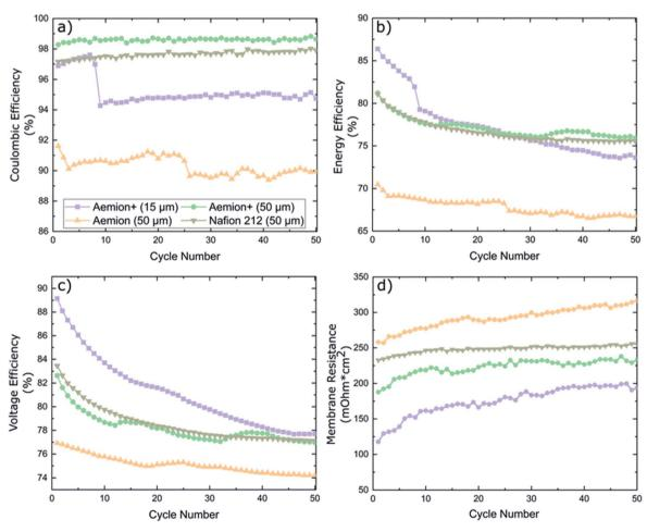
Fig. 5 Cycling data for Aemion (50 μm), Aemion+ (50 μm), Aemion+ (15 μm) and Nafion 212 (50 μm) was obtained by cycling at 100 mA cm<sup>-2</sup> with an electrode active area of 5 cm<sup>2</sup>. (a) Coulombic efficiency, (b) energy efficiency, (c) voltage efficiency and (d) membrane Ohmic resistance are reported
