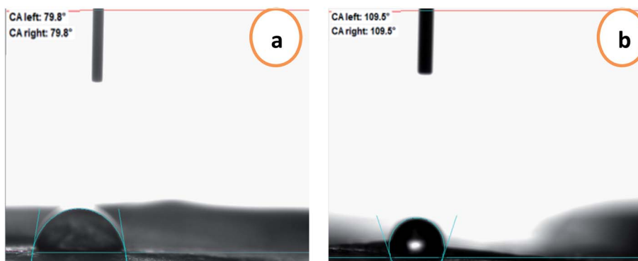
Fig. 4 Contact angle values of the chitosan (a) and chitosan–BW/PG (b) films.
