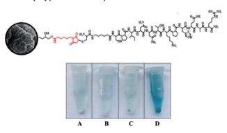
**Fig. 8** Antigen—antibody interaction assays of functionalized monolithic material. (A) Post-IV serum incubated in the absence of a monolith; (B) post-IV serum incubated with poly(GMA-co-EDMA); poly(GMA-co-EDMA)-Mhx-C-Ahx-SPINNTKPHEAR incubated with preimmune serum, PI (C) or post-IV serum (D).
