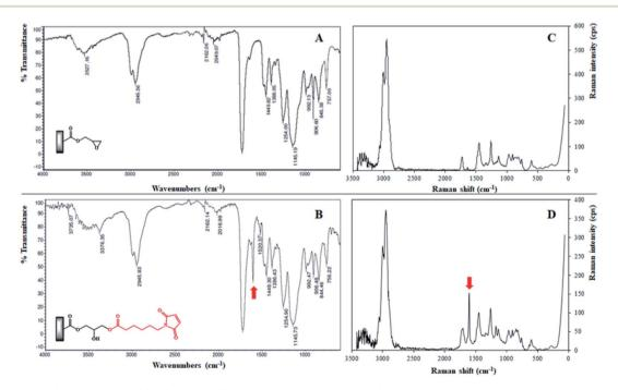
Fig. 5 Analysis of poly(GMA-co-EDMA) (top) and poly(GMA-co-EDMA)-Mhx (bottom) materials by means of FT-IR (A and B) and RAMAN (C and D). The red arrow indicates signals belonging to the maleimide group.
