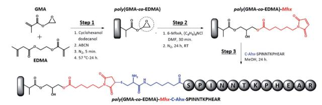
Fig. 3 General scheme for the synthesis of the organic monolithic support of poly(GMA-co-EDMA) chemically modified with a peptide. Step 1: GMA-EDMA polymerization to obtain poly(GMA-co-EDMA). Step 2: grafting of poly(GMA-co-EDMA) with 6-maleimidohexanoic acid to obtain poly(GMA-co-EDMA)-Mhx. Step 3: functionalization of poly(GMA-co-EDMA)-Mhx with a peptide containing a cysteine and 6-aminohexanoic residues and a sequence derived from L1-HPV protein.
