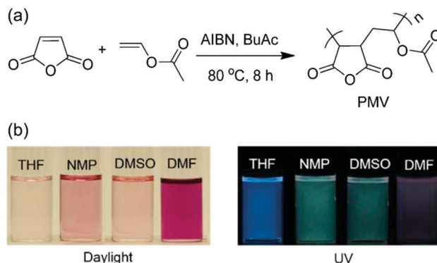
Fig. 8 (a) Synthetic Route to PMV. (b) Photographs of PMV in different solvents were taken under (left) daylight and (right) 365 nm UV light illumination. Reprinted with permission from ref. 76. Copyright 2015, American Chemical Society.
