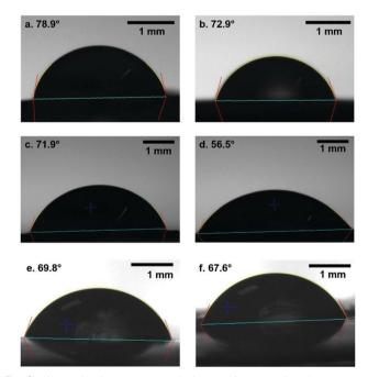
Fig. 6 Water droplet contact angle images for control and test membranes. (a) Control membrane, top-side (dense skin layer). (b) Control membrane, bottom-side (lenticular pore layer). (c) PABA-containing membrane, top-side (dense skin layer). (d) PABA-containing membrane, bottom-side (lenticular pore layer). (e) PABA-containing membrane after PABA removal, top-side (dense skin layer). (f) PABA-containing membrane after PABA removal, bottom-side (lenticular pore layer).
