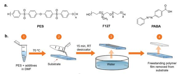
Fig. 1 (a) Chemical structures of poly(ethersulfone) (PES), Pluronic F-127 (a = 101, b = 56) (F127) and 4-(phenylazo)benzoic acid (PABA). (b) Schematic diagram of the non-solvent induced phase separation process for membrane manufacture. (1) Solution of PES, F127, and optional PABA, in DMF heated to 70 °C. (2) Solution poured onto prepared glass substrate, stored in desiccator for 15 minutes. (3) Coated substrate fully immersed in water. (4) Solid product membrane is removed from substrate
