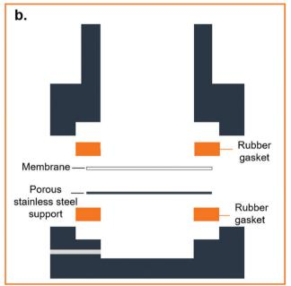
Fig. 2 (a) Photograph of the permeability testing rig in use. (b) Close-up schematic of the sample-holding chamber. A stainless steel pressure vessel is filled with water above a membrane sample. This is then pressurized using an air-line to push water through the sample. The mass of the water can be measured after a known time at a given pressure to give a flow rate
