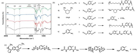
Fig. 2 (a) FT-IR spectra of the polyurea (P2-3) and polyurethane/urea (P6-7) nanocapsules. (b) Scheme for the reactions between the diamines monomers and from hydrolyzed diisocyanates, water, and diols with the toluene-2,4-diisocyanate (TDI) (c) Mechanism of the hydrolysis of isocyanate and decarboxylation of the carbamic acid in the presence of water.
