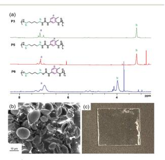
Fig. 3 (a)  $^1\text{H-NMR}$  spectra of polyurea/urethane nanocapsules (entries P3, 5 and 6) in acetone-d<sub>6</sub>: TFA (40:60). (b) SEM micrograph of polyurea microcapsules prepared by interfacial polymerization in an oil-in-water emulsion. (c) Photograph of a polyurethane coating prepared by the reaction between resorcinol and HMDI.
