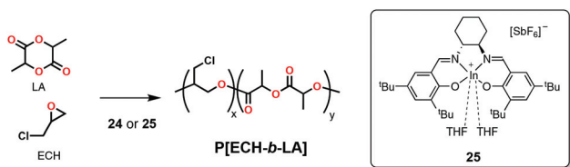
Scheme 23 Cationic indium complex active in the block copolymerization of epichlorohydrin and lactide through the simultaneous addition of monomers.
