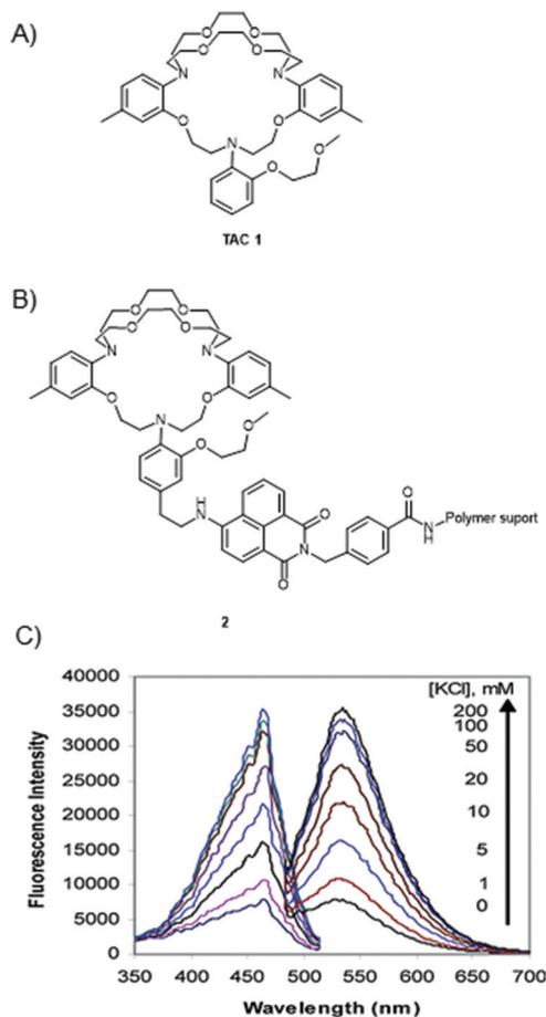
**Fig. 1** (A) Triazacryptand[2,2,3]-1-(2-methoxyethoxy) benzene (TAC). (B) He's design for an optical sensor. (C) Excitation and emission spectra of a sensor disk exposed to different potassium chloride solutions in TRIS-HEPES buffer at pH 7.40 (left, excitation spectra, fixed emission at 540 nm; right, emission spectra, fixed excitation at 470 nm. Reproduced with permission ref. 32, copyright American Chemical Society.
