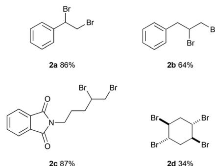
**Fig. 2** Electrochemical dibromination of alkenes in flow. Reaction conditions: alkene (0.1 M, 0.7 mmol), hydrobromic acid (48% w/w in water, 0.6 M); MeCN; 0.4  $\text{mL min}^{-1}$ , 4  $\text{F mol}^{-1}$  (257 mA); constant current; undivided cell; graphite anode (surface area: 12  $\text{cm}^2$ ); Pt coated Ti cathode.
