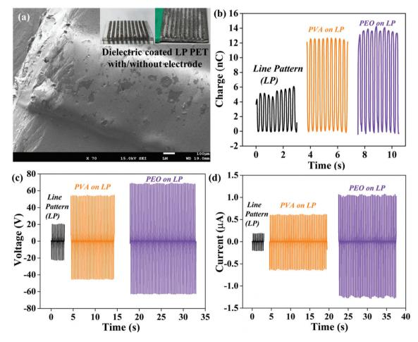
Fig. 3 (a) Photographic image of the dielectric coated with and without electrode LP PET (b) transfer charges of single and double-layered TENG (c) and (d)  $V_{OC}$  and  $I_{SC}$  measurement of DL<sub>1</sub> and DL<sub>2</sub> TENG devices with the fixed operational parameters i.e., frequency of 5 Hz, CS distance 4 mm, and a force of 50 N.
