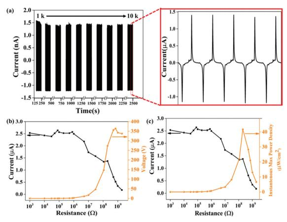
Fig. 5 (a) Endurance evaluation of  $I_{sc}$  for the DL<sub>2</sub> device operated up to 10 000 cycles with a force of 50 N, frequency of 4 Hz, and CS distance of 4 mm; the inset images show that performance at the middle of the endurance operation evaluation and peak degradation analysis. (b)  $V_{oc}$  and  $I_{sc}$ across the different load resistance, and (c) Instantaneous max power density measurement with the different load resistance.
