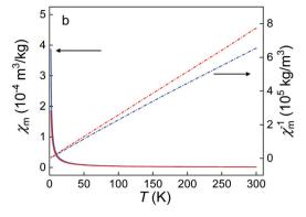
Fig. 2 (a) Magnetization curves of GdF<sub>3</sub>@EG (blue) and GdF<sub>3</sub>@PSSMA nanoparticles (red) at 2 (solid line) and 300 K (dot line) and (b) temperature dependence of mass magnetic susceptibility ( $\gamma_m$ ; solid line) and inverse mass magnetic susceptibility of particles ( $\gamma_m^{-1}$ ; dot line) measured at cooling in the applied magnetic field of 0.1 T.
