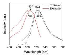
Fig. 4 Photoluminescence spectra of PSDA-A488 (dotted line) and  $GdF_3@PSSMA-PSDA-A488$  nanoparticles (solid line).
