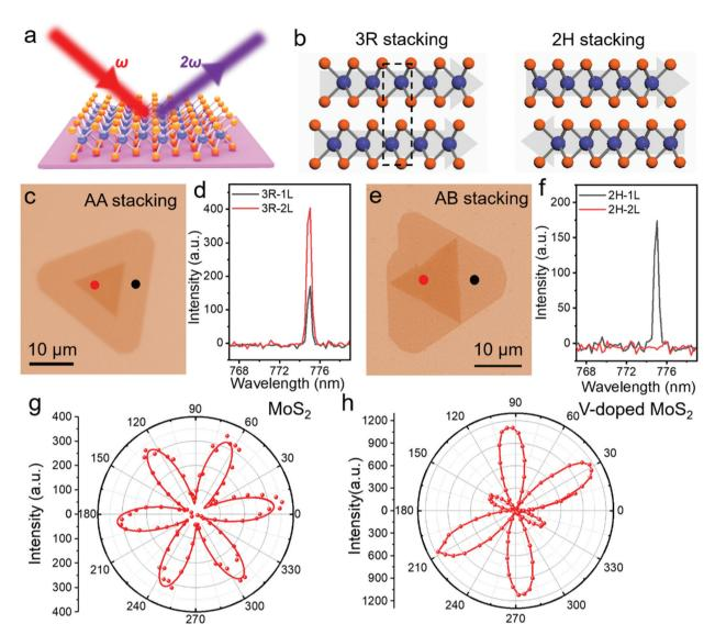
Fig. 4 (a) Schematic diagram of SHG process. (b) Side view of bilayer 3R and 2H phase  $MoS_2$  with different stacking order. (c and e) Optical images of  $MoS_2$  with 3R and 2H stacking. (d and f) Layer number-dependent SHG response 3R and 2H phase V-doped  $MoS_2$ . (g and h) Angular-dependent SHG intensity of monolayer  $MoS_2$  and V-doped  $MoS_2$ .
