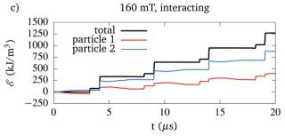
Fig. 8 (a) Hysteresis loops for particles, excited with an sinusoidal externally applied magnetic field with amplitudes of 75 mT (red lines) and 160 mT (blue lines). (b) and (c) Dissipated heat by individual particles as function of time for 10 periods of the field excitation with amplitude 75 mT [panel (b)] and 160 mT [panel (c)], respectively. These figures correspond to the cases highlighted with filled dots in Fig. 6.
