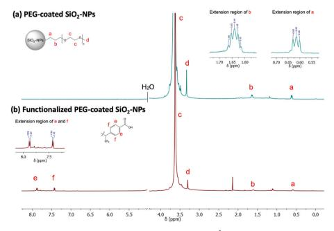
Fig. 3 Stacked <sup>1</sup>H spectra of empty PEG-coated silica nanoparticles (D<sub>2</sub>O, 500 MHz). <sup>1</sup>H NMR spectrum (a) before and (b) after photografting (365 nm, 45 min) and purification step. NMR peak at 2.2 ppm (bottom spectrum) arises from acetone.
