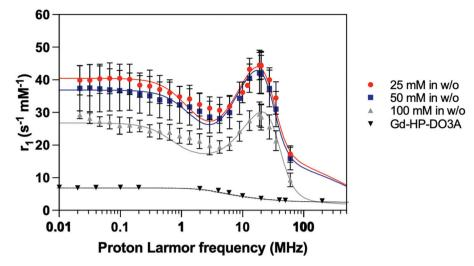
Fig. 5 NMRD profiles (T = 37 °C) obtained for the paramagnetic complexes entrapped on PEG-coated SiO<sub>2</sub>-Gd-NPs (16, 18 and 25 nm) as a result of [Gd-HP-DO3A] in w/o procedure (triangles, squares and squares on edge, respectively) and free Gd-HP-DO3A complex (circles) in aqueous solution. Longitudinal  $(r_1)$  relaxometric measurements plots are normalized per paramagnetic gadolinium ion concentration  $(s^{-1} \text{ mM}^{-1})$ .
