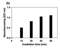
Fig. 2 UV irradiation time study. (a) UV spectra after purification and (b) plot result of the linker absorbance (233 nm) on PEG-coated SiO<sub>2</sub>-NPs normalized per mg of particles for different time of exposure.
