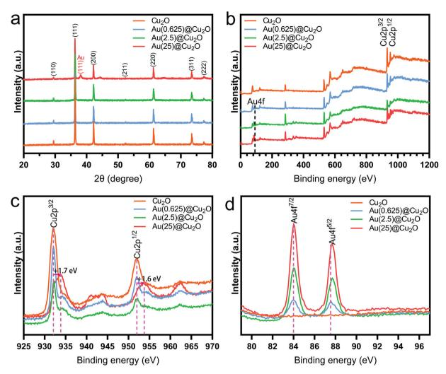
Fig. 2 The phase structure and chemical composition of  $Cu_2O$  and  $Au@Cu_2O$  nanocubes. (a) XRD patterns. (b) XPS spectra, with the survey scan ranging from 0 to 1200 eV. (c) XPS spectrum survey of the Cu 2p band. (d) XPS spectrum survey of the Au 4f band.
