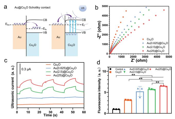
Fig. 3 Evaluation of sonocatalytic activity and ROS generation ability. (a) Schematic diagram of a Schottky contact between Au and Cu<sub>2</sub>O. (b) Electrochemical impedance spectra of different samples. (c) US current curves of different samples under US stimulation. (d) ROS generation abilities of different samples detected by the fluorescence intensity of DCF. n = 3 independent experiments per group; \*P < 0.05 and \*\*P < 0.01.
