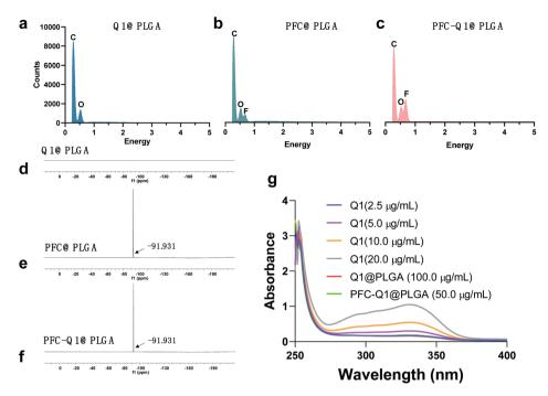
Fig. 2 (a-c) EDS of three nanoparticles. (d-f)  $^{18}$ F MRS spectra of three nanoparticles. (g) UV spectra of Q1 and nanoparticles at gradient concentrations. The curves of Q1@PLGA (100.0  $\mu$ g mL $^{-1}$ ) and PFC-Q1@PLGA (50.0  $\mu$ g mL $^{-1}$ ) were overlapped with that of Q1 (2.5  $\mu$ g mL $^{-1}$ ).
