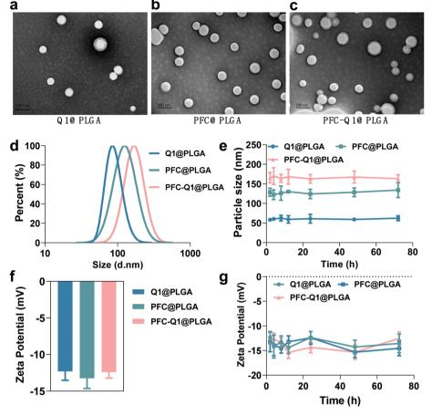
Fig. 1 Characterization of nanoparticles. (a–c) TEM images of Q1@PLGA, PFC@PLGA and PFC-Q1@PLGA (scale bar: 100 nm). (d) Hydrodynamic sizes of three nanoparticles measured by DLS. (e) Colloidal stability of nanoparticles in DMEM containing 10% FBS. (f) Zeta potentials of three nanoparticles. (g) Stability of nanoparticles in water.
