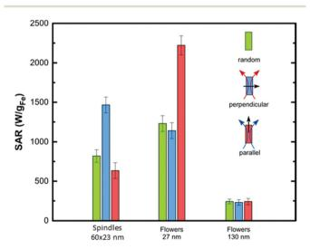
**Fig. 8** SAR values before (green) and after orientation attempted (perpendicular, blue; and parallel, red) under AC field (24 kA  $\rm m^{-1}$ , 765 kHz) for small spindles, small and large nanoflowers stabilized in agarose compared to their random initial state.
