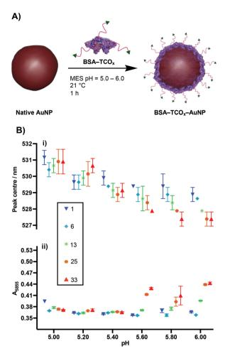
Fig. 2 (A) Schematic representation of physisorption of BSA-TCO<sub>x</sub> onto AuNPs. (B) UV-Vis data of physisorption of BSA-TCO<sub>x</sub> to 40 nm citrate-capped AuNPs (N = 3, mean  $\pm$  SD); (i) plasmon peak centre vs. pH, (ii) measure of flocculation ( $A_{585}$ ) vs. pH of BSA-TCO<sub>x</sub>-AuNP particles subjected to high salt concentration. The numbers in the legend (square box) represent the TCO: BSA ratio.
