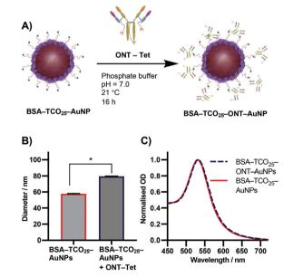
Fig. 6 (A) Schematic representation of the iEDDA reaction between BSA-TCO $_{25}$ -AuNPs and ONT-Tet. (B) DLS data showing the diameter of BSA-TCO $_{25}$ -AuNPs after addition of ONT-Tet. Data plotted as mean  $\pm$  SD (N=3). Statistical significance \* (P=0.0001) was determined using an unpaired t-test. (C) UV-Vis spectra comparing BSA-TCO $_{25}$ -AuNPs and BSA-TCO $_{25}$ -ONT AuNPs.
