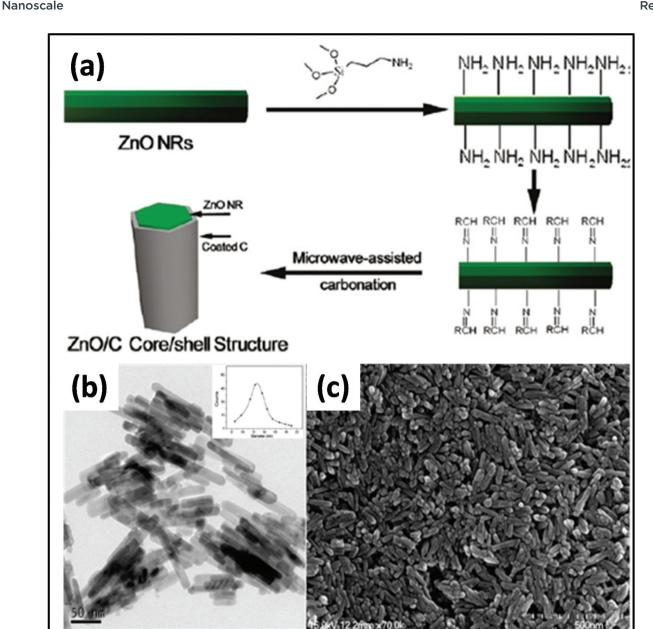
Fig. 10 (a) Schematic diagram showing the synthesis of carbon-coated ZnO. (b) TEM (inset: average size distribution of 200 rods) and (c) SEM images of ZnO nanorods.<sup>204</sup> Reprinted (adapted) with permission from ref. 204, copyright (2009), the American Chemical Society.
