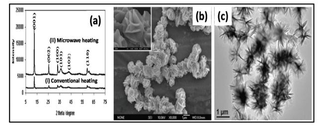
Fig. 8 (a) XRD pattern of  $\alpha$ -Ni(OH)<sub>2</sub> synthesized by (i) conventional heating method and (ii) MW heating method. (b) SEM image of  $\alpha$ -Ni(OH)<sub>2</sub> and (c) TEM image of α-Ni(OH)<sub>2</sub>.<sup>179</sup> Reprinted (adapted) with permission from ref. 178 and 179, copyright (2008 and 2010), the American Chemical
