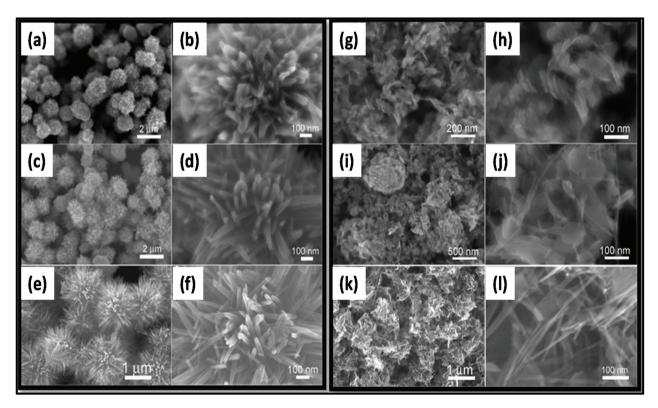
Fig. 15 SEM images of  $MnO_2$  prepared at (a, b, g, and h) 5 min, (c, d, i, and j) 10 min, and (e, f, k, and l) 30 min under (a-f) acidic condition and (g-l) neutral condition.<sup>257</sup> Reprinted (adapted) with permission from ref. 257, copyright (2013), Elsevier B.V. All rights reserved.
