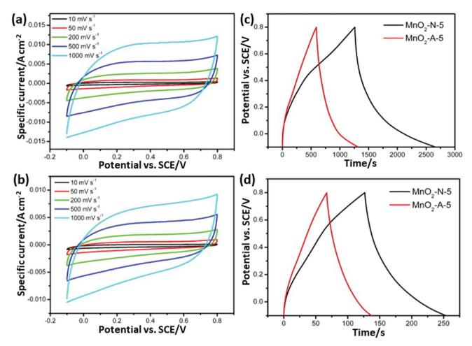
Fig. 16 (a and b) CV curves of  $MnO_2-N-5$  and  $MnO_2-A-5$  at different scan rates and (c and d) charge/discharge curves of  $MnO_2-N-5$  and  $MnO_2-A-5$  at current densities of 0.2 A  $g^{-1}$  and 1 A  $g^{-1}$ , respectively. Reprinted (adapted) with permission from ref. 257, copyright (2013), Elsevier B.V. All rights reserved.
