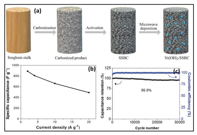
Fig. 18 (a) Synthesis of Ni(OH)<sub>2</sub>/sorghum stalk biomass carbon, (b) specific capacitance of Ni(OH)<sub>2</sub>/sorghum stalk biomass carbon composite and (c) cyclic property and columbic efficiency of Ni(OH)<sub>2</sub>/sorghum stalk biomass carbon composite. Reprinted (adapted) with permission from ref. 267, copyright (2020), Elsevier B.V. All rights reserved.
