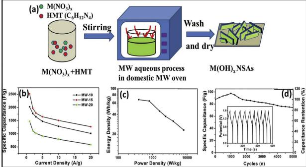
Fig. 17 (a) Schematic of MW-assisted synthesis of layered metal hydroxide nanosheet arrays, (b) specific capacitance vs. current density of Ni(OH)<sub>2</sub> nanosheet arrays, (c) Ragone plot and (d) cycle curves of Ni(OH)<sub>2</sub> nanosheet arrays//activated carbon aqueous hybrid supercapacitor. Reprinted (adapted) with permission from ref. 265, copyright (2019), Elsevier B.V. All rights reserved.
