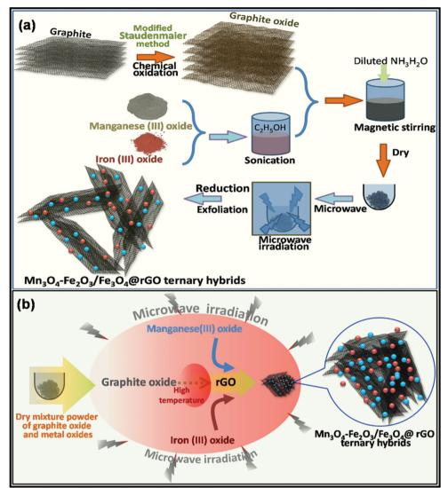
Fig. 13 Schematic presentation of the (a) synthesis process and (b) mechanism of MW-assisted formation of  $Mn_3O_4$ -Fe $_2O_3$ /Fe $_3O_4$ @rGO ternary hybrid. Reprinted (adapted) with permission from ref. 222, copyright (2020), Elsevier B.V. All rights reserved.
