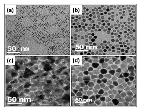
Fig. 6 TEM images of  $Fe_3O_4$ : effect of using different compositions and times of MWI. (a) 4 nm and (b) 20 nm prepared using the same ratio of oleic acid to oleylamine (1:1) at different MW times (6–8 min and 15–18 min, respectively). (c) Triangular and prism shapes and (d) quasi cubes and triangular shapes prepared using oleic acid to oleylamine ratios of 2:1 and 3:1, respectively. (adapted) with permission from ref. 161, copyright (2013), Springer. All rights reserved.
