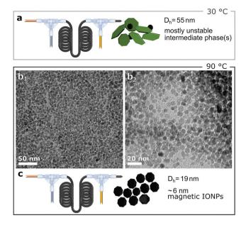
Fig. 4 (a) Schematic of flow synthesis with co-precipitation performed at 30 °C. (b<sub>1-2</sub>) TEM images of IONPs synthesised with co-precipitation performed at 90 °C,  $D_{TEM} = 6.1 \pm 0.9$  nm. (c) Schematic of flow synthesis with co-precipitation initiated at 90 °C. Fig. S5† shows the particle size distribution. For both temperatures, quenching was performed at 5 s.
