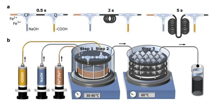
Fig. 1 Schematic of (a) precisely-timed quenching (Q) of particle growth after 0.5 s, 2 s and 5 s after initiation of co-precipitation (CP) and (b) multistage flow reactor to initiate co-precipitation (step 1), quenching and stabilisation (step 2, here after 0.5 s) and aging (step 3).
