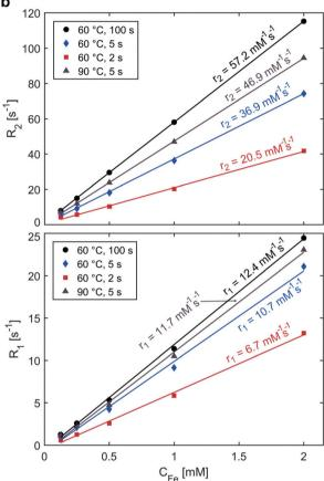
Fig. 5 (a) IONP solutions synthesised with quenching times of 100, 5 and 2 s at 60 °C and 5 s at 90 °C (from left to right) selected for MRI contrast performance evaluation. (b) Relaxation rates  $R_2$  (transversal, top) and  $R_1$  (longitudinal, bottom) vs. iron concentration in the (consecutively diluted) dialysed samples ( $C_{\text{Fe}}$ ) to determine  $r_1$  and  $r_2$  (i.e., the slope) for IONPs synthesised at co-precipitation temperatures and quenching times as indicated.
