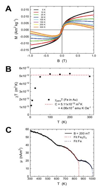
Fig. 5 Magnetic characterization of AuFe NPs. (A) Hysteresis loops recorded at various temperatures between 5 K and 300 K. (B)  $\gamma T$  (T) plot after subtraction of the Au diamagnetic component for the evaluation of the Curie constant; (C) high-temperature total magnetic moment of another sample at B = 200 mT. Two ordering temperatures are obtained as identified by the fits for Fe<sub>3</sub>O<sub>4</sub> and Fe using mean field models while the dip at 600 K is due to diffusion.
