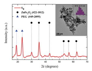
Fig. 1 All the peaks of the XRD pattern are well-matched with the standard JCPDS data of ZnFe<sub>2</sub>O<sub>4</sub>, while the two distinct peaks at 19° and 23° confirm the presence and crystallization of PEG on the surface. The bright-field TEM image of the sample (S<sub>4</sub>) clearly shows nearly spherical nanoparticles covered by PEG.
