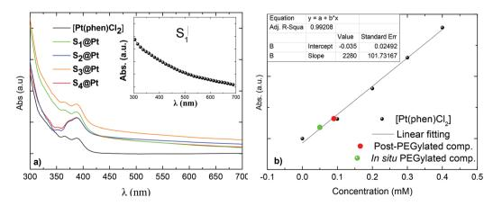
Fig. 3 (a) Absorption spectra of the composites and the Pt-complex diluted in DMSO, (inset) indicative spectrum of the primary zinc ferrite MNPs coated by propylene glycol ( $S_1$ ) and (b) calibration curve (black circles) and amount of Pt-complex of post-PEGylated (red circle) and *in situ* PEGylated (green circle) composites.
