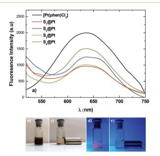
Fig. 4 (a) Solid-state fluorescence emission spectra ( $\lambda_{\rm ex}$  = 400 nm) of the composites and the Pt-complex. Digital pictures of (b) aqueous solution of the composite S<sub>3</sub>@Pt under daylight, (c) aqueous solution of the composite under magnetic field and under daylight, (d) and (e) corresponding pictures under UV excitation ( $\lambda_{\rm exc}$  = 365 nm).
