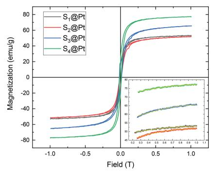
Fig. 5 The magnetization *versus* the magnetic field, M(H), dependence for the MNP samples after different degrees of polyol functionalization. The magnetization curves were obtained at 300 K. The inset is the fitted magnetization-field data with the law of approach described by eqn (1). The symbols, following the same color indexing to the entire M(H) curves, are the experimental data and the yellow lines are the fittings.
