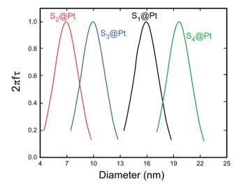
Fig. 7 Dependence of the factor  $2\pi f\tau$  on the MNP diameter for the whole set of samples. This maximum corresponds to the resonant size of our MNPs for the working frequency of 765 kHz. The relaxation time  $\tau$ was calculated by taking into account the Néel and Brown moment relaxation mechanisms that were obtained from egn (3) and (7), respectively.
