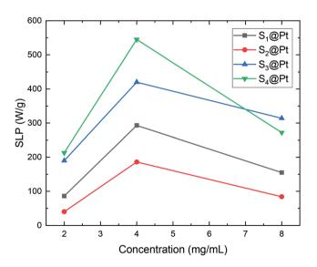
Fig. 10 SLP values of samples S<sub>1</sub>@Pt, S<sub>2</sub>@Pt, S<sub>3</sub>@Pt and S<sub>4</sub>@Pt for the three different concentrations (2, 4 and 8 mg mL<sup>-1</sup>) used in magnetic hyperthermia experiments.
