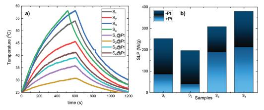
Fig. 6 (a) Heating sequence curves of the PEGylated MNPs and hybrid composites after 600 s of MH treatment and 600 s of sample cooling. The concentration was the same for all samples and equal to 2 mg mL<sup>-1</sup>, (b) SLP values of samples before (–Pt) and after (+Pt), the absorption of the complex [Pt(phen)Cl<sub>2</sub>]. An obvious reduction in SLP is observed for all samples.
