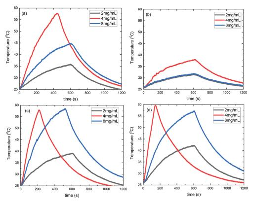
Fig. 9 Experimental curves of heating sequence during MH of (a) S1@Pt, (b) S2@Pt, (c) S3@Pt and (d) S4@Pt at three different concentration values namely 2, 4 and 8 mg mL<sup>-1</sup>. AMF amplitude and frequency were set to 24 kA m<sup>-1</sup> and 765 kHz respectively. The concentration value of 4 mg mL<sup>-1</sup> presented the higher heating rate verifying theoretical estimations.
