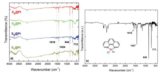
Fig. 2 FT-IR spectra of (a) hybrid magneto-fluorescent composites in comparison with the (b) synthesized platinum complex, [Pt(phen)Cl<sub>2</sub>].
