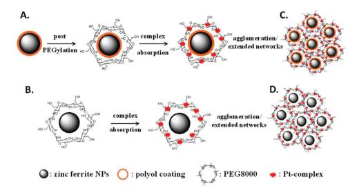
Scheme 1 Illustration of the design of hybrid nano-molecular composites. Firstly, post (1) or in situ (2) PEGylation was promoted on particles' surface and, finally, the Pt-complex was absorbed into the hydrophobic polymer's chains.
