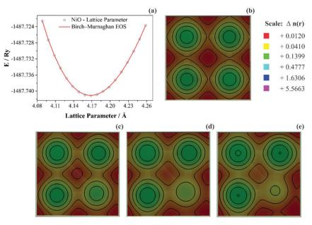
Fig. 7 (a) NiO equation of state (EOS) from DFT-data and Birch-Murnaghan fitting, (b) NiO charge density map using Ni-0.0 Å displacement, (c) Ni-0.01 Å displacement, (d) Ni-0.02 Å displacement, and (e) Ni-0.03 Å displacement.
