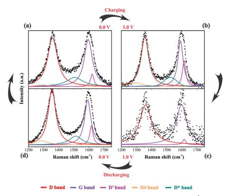
Fig. 6 Raman spectra of the electrode/electrolyte interface under cyclic voltammetry at scan rate  $0.15 \text{ mV s}^{-1}$  from (a) 0 V to (b) 1 V during charge and from (c) 1 V to (d) 0 V during discharge. Spectra intensities are normalized from 0 to 1 in the 1200 to 1750 cm<sup>-1</sup>. Electrodes were housed in an El Cell filled with 80 µL of a 1 M Li<sub>2</sub>SO<sub>4</sub> aqueous solution. Deconvolution considered five bands as described in Fig. 1(d).
