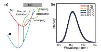
**Fig. 8** (a) A simplified model for the zero-thermal-quenching due to structural defects. (b) Temperature-dependent emission spectra of Na<sub>3</sub>Sc<sub>2</sub>(PO<sub>4</sub>)<sub>3</sub>:Eu (divalent, 0.7%) phosphors under 370 nm excitation in the temperature range of 25–200 °C. Reproduced with permission from ref. 104. Copyright 2017, Nature Publishing Group.
