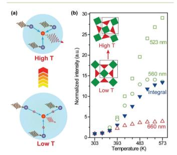
Fig. 7 (a) Thermal promotion of energy delivery to activator ions by lattice contraction in negative thermal expansion crystals. (b) Normalized emission intensities of  $Yb_2W_3O_{12}$ :Er (6%) nanocrystals as a function of temperature. Inset: schematic of the lattice contraction and distortion as the temperature increases. Adapted with permission from ref. 101. Copyright 2019, Wiley-VCH.
