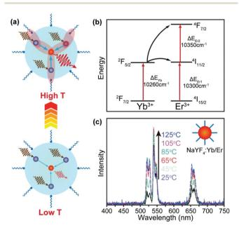
Fig. 6 (a) Thermal activation of phonon-assisted energy transfer. (b) Mismatch of energy levels between  $Yb^{3+}$  and  $Er^{3+}$  ions, illustrating the need for phonon participation in the energy transfer process. (c) Temperature-dependent upconversion emission spectra of NaYF<sub>4</sub>:Yb/Er (20/2%) UCNPs (24 nm) in the temperature range of 25-125 °C. Reproduced with permission from ref. 79. Copyright 2014, American Chemical Society.
