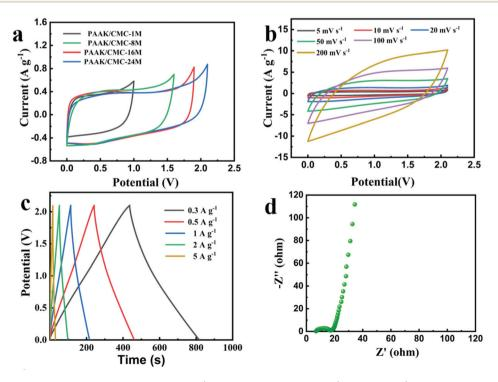
Fig. 3 Voltage windows of PAAK/CMC-1, 8, 16, 24 M at 5 mV s<sup>-1</sup> (a), CV curves from 5 mV s<sup>-1</sup> to 200 mV s<sup>-1</sup> (b), GCD profiles from 0.3 A g<sup>-1</sup> to 5 A g<sup>-1</sup> (c) and EIS (d) of the NG//NG quasi-solid-state supercapacitor with the PAAK/CMC-24 M polyelectrolyte hydrogel.
