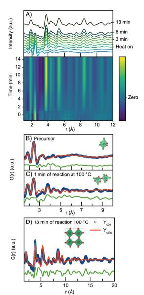
Fig. 8 (A) Time resolved PDFs collected at ambient pressure at temperature 100 °C. (B) Refinement of the precursor PDF using a single [NbCl<sub>4</sub>O<sub>2</sub>] octahedra. (C) Refinement of the PDF collected at 1 min of reaction with a polyhedral cluster of [NbCl<sub>6–x</sub>O<sub>x</sub>] octahedra. (D) Refinement of PDF collected after 13 min of reaction using the ReO<sub>3</sub> structure.
