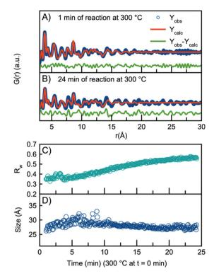
Fig. 3 PDF fit using the H-Nb<sub>2</sub>O<sub>5</sub> structure to the data collected (A) after 1 min of reaction and (B) 24 min of reaction. (C) Rw values obtained from sequential refinement with H-Nb<sub>2</sub>O<sub>5</sub> plotted as a function of time. (D) The refined crystallite size plotted as a function of time.
