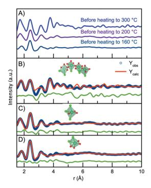
Fig. 7 (A) PDFs collected for the precursor for each of the three experiments. (B) PDF fit to the data obtained for the 300 °C precursor, using a chain of [NbCl<sub>6-x</sub>O<sub>x</sub>] octahedra. (C) PDF fit to the data obtained for the 200 °C precursor, using a single [NbCl<sub>3</sub>O<sub>3</sub>] octahedra. (D) PDF fit to the data obtained for the 160 °C precursor, using a single [NbCl<sub>3</sub>O<sub>3</sub>] octahedra.
