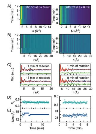
Fig. 6 (A) Time resolved XRD data and (B) PDFs obtained from experiments conducted at 160 °C and 200 °C. (C) PDF fit of data collected 1 min into the reaction, and at the end of the experiments using  $H-Nb_2O_5$  as the structure model. (D)  $R_w$  values obtained from sequential refinements with the H-Nb<sub>2</sub>O<sub>5</sub> model plotted as a function of time. (E) The refined crystallite size (sp-diameter) plotted as a function of time.
