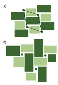
Fig. 4 (A) Idealized representation of  $H-Nb_2O_5$ . Dark green circles represent tetrahedral sites and the dark and light green squares represent  $ReO_3$  type blocks. The black rhombus illustrates the unit cell of the  $H-Nb_2O_5$ . (B) A distorted version of  $H-Nb_2O_5$  with several different block sizes and no systematic ordering.
