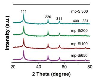
Fig. 1 Powder XRD patterns of mp-Si NPs prepared using a single heating step magnesiothermic reduction process at 650 °C for 3 h (mp-Si650) and two heating steps with the second annealing temperature of 100 (mp-Si100), 200 (mp-Si200), and 300 °C (mp-Si300).
