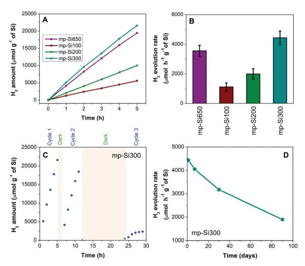
Fig. 4 (A) H<sub>2</sub> evolution profiles of different mp-Si NPs under broadband illumination, (B) H<sub>2</sub> evolution rates of mp-Si NPs, (C) photocatalytic cyclability of mp-Si300 NPs, and (D) the change in the H<sub>2</sub> evolution rate of mp-Si300 NPs with catalyst aging.
