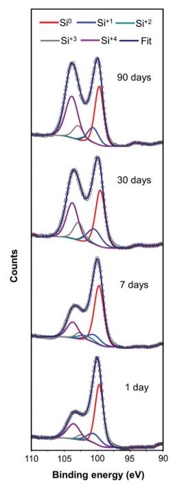
Fig. 5 High resolution XP spectra of the Si 2p region of mp-Si300 NPs at different times after the synthesis and storage under ambient conditions. For clarity, only  $2p_{3/2}$  peaks of different oxidation states are shown.
