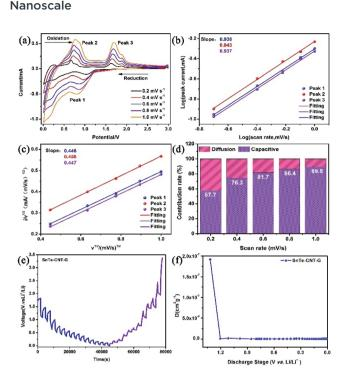
Fig. 5 (a) CV curves obtained at different scan rates. (b) The corresponding  $\log(i)$  versus  $\log(v)$  plots and (c) the corresponding  $i/v^{1/2}$  versus  $v^{1/2}$  plots of the SnTe-CNT-G electrodes. (d) The normalized ratio of the capacitive- and diffusion-controlled contributions at different scan rates. GITT curves of the SnTe-CNT-G electrode (e) and their Li<sup>+</sup> diffusion coefficient for the initial discharge states (f).
