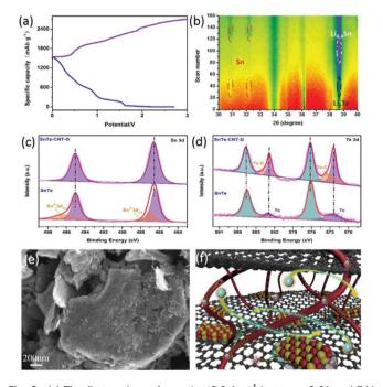
Fig. 6 (a) The first cycle performed at 0.2 A  $g^{-1}$  between 0.01 and 3 V. (b) The contour plots of the *in situ* XRD patterns obtained for the SnTe-CNT-G anodes during the initial cycle. XPS core-level spectra of (c) Sn 3d and (d) Te 3d for the SnTe-CNT-G and SnTe electrodes at a current density of 200 mA  $g^{-1}$  after 100 cycles. (e) SEM images of the SnTe-CNT-G electrode at 200 mA  $g^{-1}$  after 100 cycles. (f) Schematic diagram of the storage mechanism of the SnTe-CNT-G anode.
