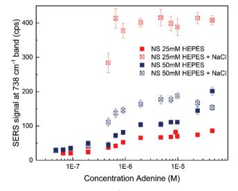
**Fig. 3** SERS signal of the 738 cm<sup>-1</sup> band in the spectrum of adenine as a function of adenine concentration for nanostars synthesized with different HEPES concentration in the presence and absence of NaCl. Each signal value was obtained by averaging 30 spectra; the error bars represent the standard deviation.
