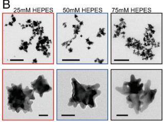
Fig. 1 (A) UV-vis-NIR spectra of gold nanostars synthesized with different HEPES concentrations. Maxima assigned to plasmon resonances are labeled for each nanostar condition. The maximum at 533 nm is common to all the spectra. (B) TEM micrographs of the nanostars. Color code is maintained. Scale bars: upper row 200 nm, lower row 20 nm
