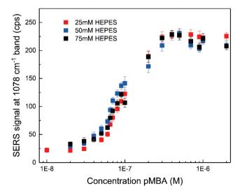
Fig. 2 SERS signal of the 1078 cm<sup>-1</sup> band in the spectrum of pMBA as a function of pMBA concentration for nanostars synthesized with different HEPES concentration. Each signal value was obtained by averaging 30 spectra and the error bars represent the standard deviation.
