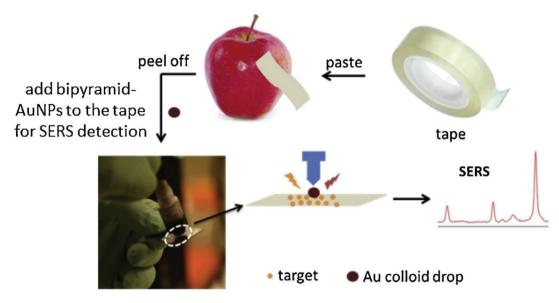
Fig. 4 Detection of pesticides using SERS substrates. The schematic shows the use of modified adhesive tape modified with bipyramid-gold nanoparticles (AuNPs) as a SERS sensor for pesticide residue detection on the surface of fruit peels. Reproduced with permission from ref. 51. Copyright 2019, Elsevier.
