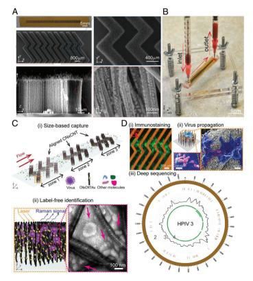
Fig. 10 Schematic of the working principle of VIRRION platform, including (A) images of aligned CNTs decorated with gold nanopaticles and (B) assembled VIRRON device, (C) illustration of virus capture and label-free Raman identification, and (D) on-chip analysis and enrichment of virus for NGS. Reprinted with no changes from ref. 122, image licensed under http://creativecommons.org/licenses/by/4.0, /.
