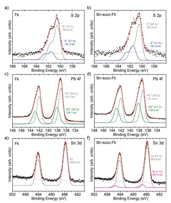
Fig. 3 XPS spectra of S, Pb and Sn core levels for (a-c) the control Fk material and (d-f) Bn-succ-Fk.
